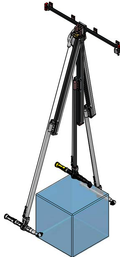
SLIDER 50 compact PC with inclinometer + lazer coders on horizontal rail
